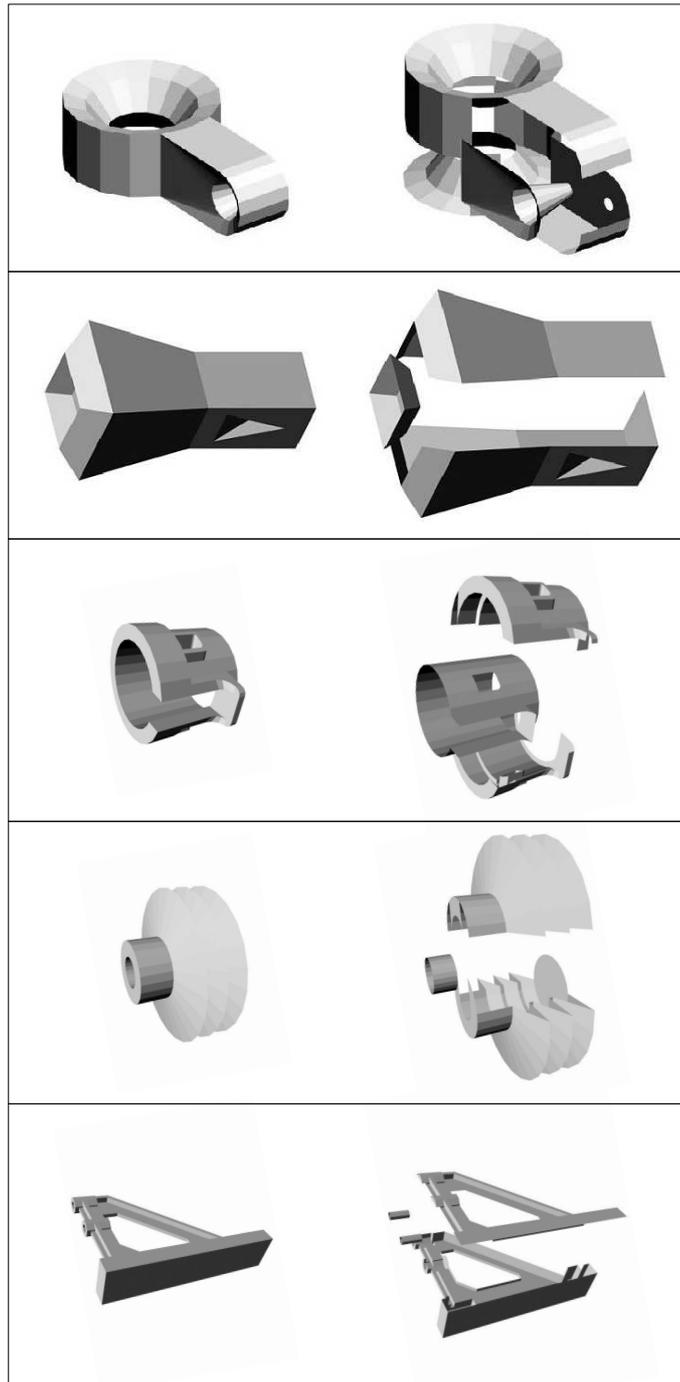
Figure 6: Objects and their boundary partitions into three groups by the implementation of our algorithm. The first two are artificial objects. The next three are a part of a camera body, a screw, and a wall bracket in order.
