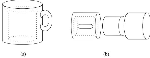
Figure 1: (a) A coffee mug is unattainable using a 2-part cast. (b) By incorporating a side core, the cavity of the coffee mug can be manufactured.
