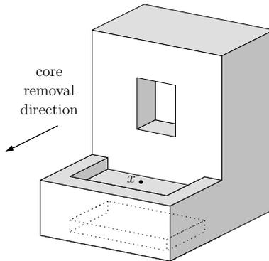
Figure 3: An object with a small hole in the middle of the vertical wall, and bigger holes on the top and bottom face of the horizontal leg. It can be produced using a 2-part cast with a side core if the side core is removed first. Consider a point  $x$  in the middle of the hole on the horizontal leg. It must be removed vertically upward, otherwise it intersects the object. But if we remove  $x$  vertically upward, we run into the swept volume of the side core, which violates our assumption.
