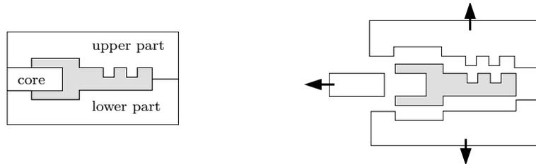
Figure 2: The casting process with a side core is illustrated in 2D.
